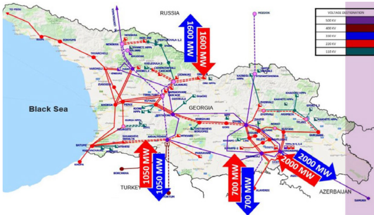
CHART 8. ABILITIES FOR CAPACITY FLOW OF GEORGIA'S TRANSMISSION GRID FOR 2033 (GEORGIAN STATE ELECTROSYSTEM).
